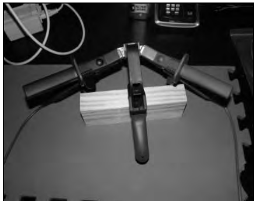
Figure 5. Solid copper plates were adhered to a non-conductive plastic clamp to which roughly five pounds of force was applied securing each wafer in-between the copper plates so that the copper plate was larger than the wafer sample to ensure that the entire wafer was exposed to the electrical current.
