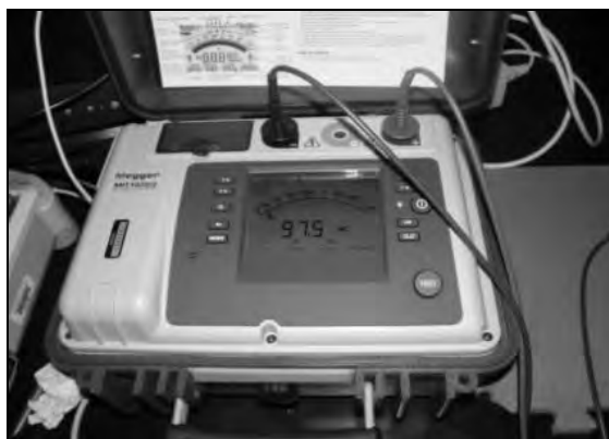
Figure 3. Resistance measurements were made using a Meger MIT 102/2 recording ohms using 1-10,000 Volts over a period of one minute.
